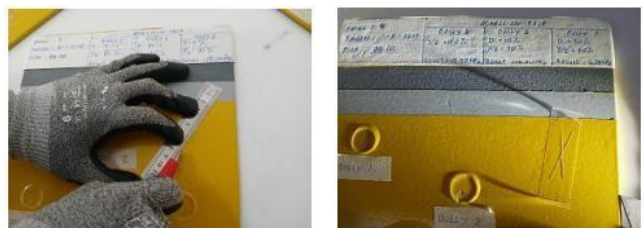
Figure 5. X-Cut Tape Test Process
