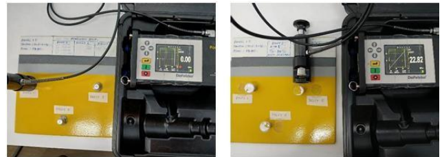
Figure 4. Pull-off adhesion test process
