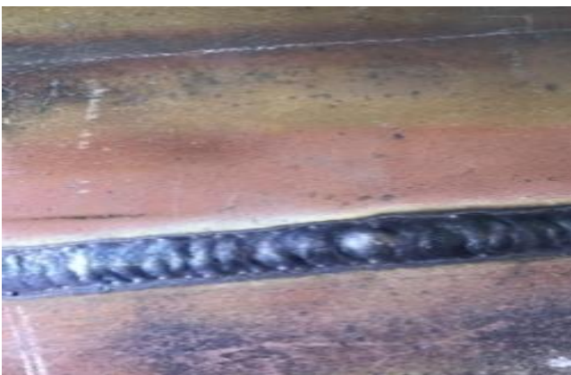
Figure 4. Welding results initial heating 200°C
