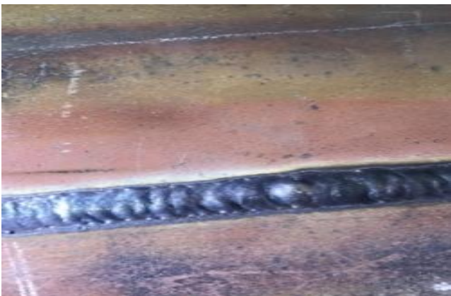
Figure 3. Welding results initial heating 100°C
