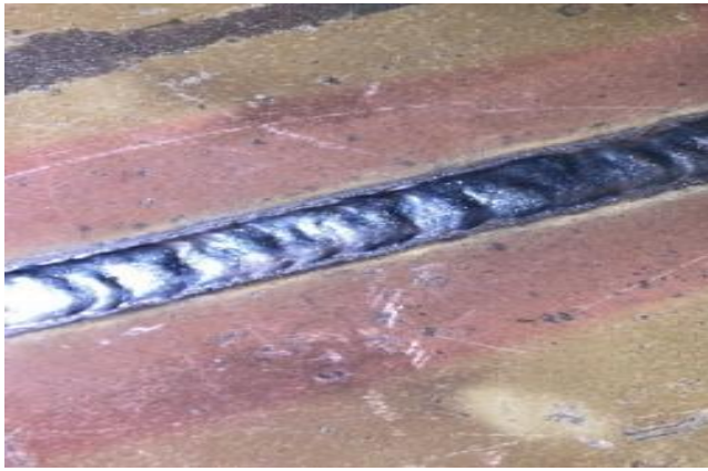
Figure 2. Welding results without preheating
