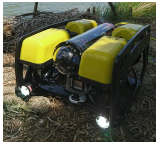
Figure1. Modeling ROV Surovotic Indonesia
